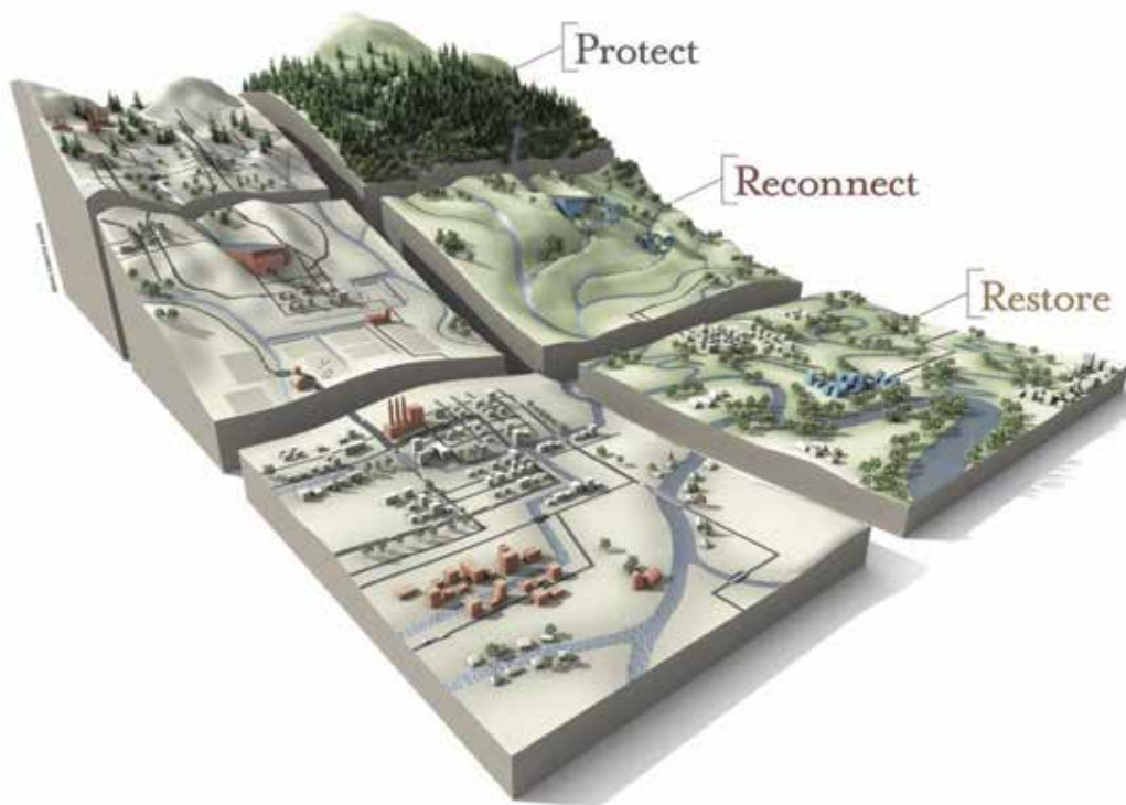
Figure 1. Graphic depicts watershed-scale adaptation strategy consisting of protecting headwater sources of cold water, reconnecting the fragmented stream network, and restoring the mainstem and valley bottom habitats. Illustration courtesy of Bryan Christie Design and Trout Unlimited.
