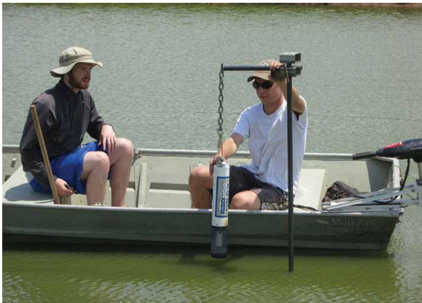
Figure 2. Graduate students John Farrelly (left) and Christopher Laskodi (right) at the Aquaculture and Fisheries Center, University of Arkansas–Pine Bluff, put a data sonde in a commercial Channel Catfish pond to monitor DO and related water quality in eastern Arkansas. Photo credit: Yushun Chen.
