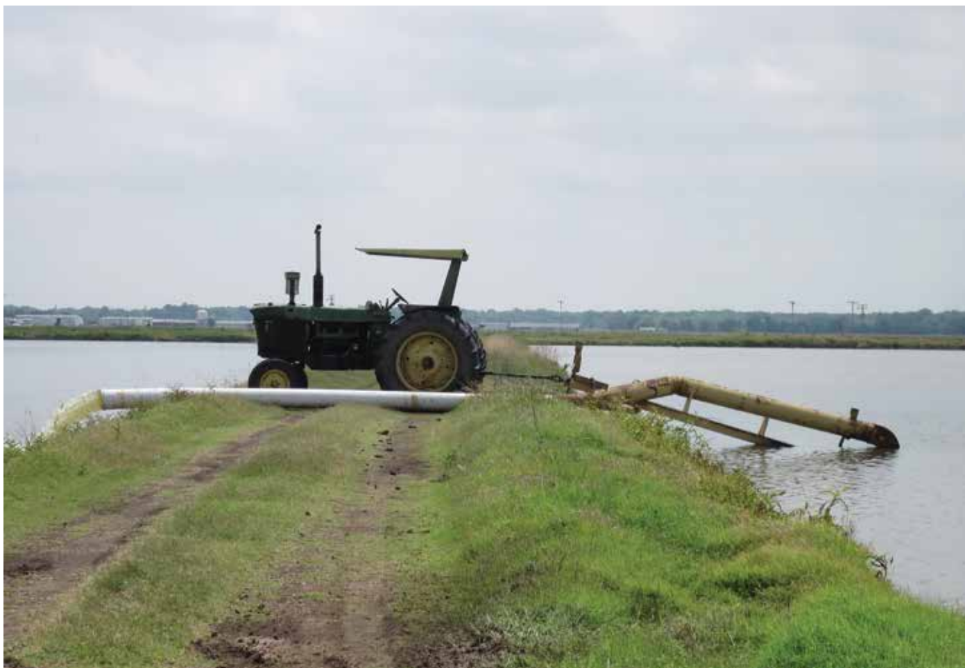
Figure 3. Draining a bait fish pond by pumping the pond water from one pond to another pond in a fish farm in east Arkansas. Photo credit: Yushun Chen.
