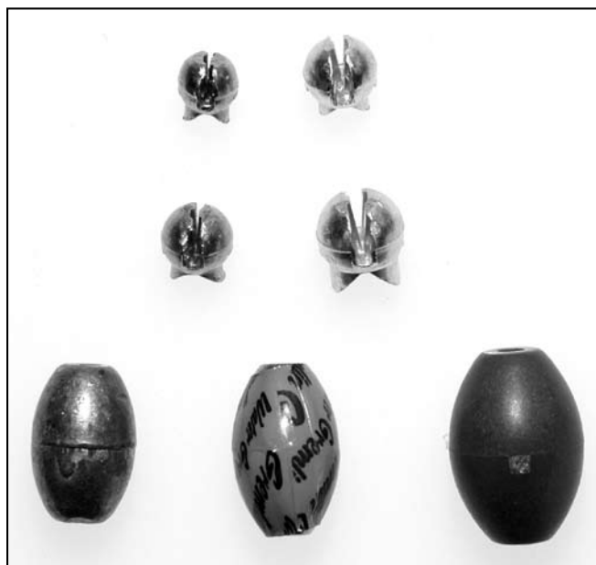
Figure 1. Relative sizes of sinkers manufactured from different materials. Top row: 0.1 oz lead and tin split shot. Middle row: 0.2 oz lead and tin split shot. Bottom row: 0.8 oz lead, bismuth, and plastic-iron composite egg sinkers. Sinkers courtesy of Water Gremlin.
