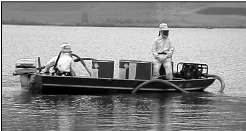
Figure 8. 16-foot John boat fitted with high pressure pump, aspirator system and 4-200 lb barrels of powdered rotenone.
